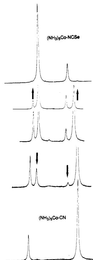
Figure 1. ^1\text{H} NMR spectra for the reaction between [(\text{NH}_3)_5\text{Co-NCSe}]^{2+} and \text{CN}^- in \text{Me}_2\text{SO-}d_6 at 25^\circ\text{C} .
